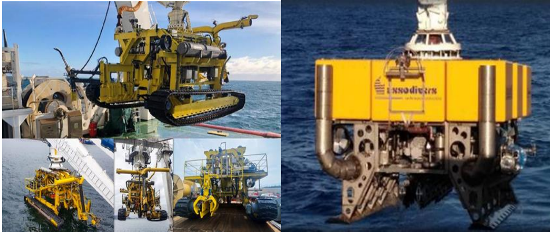
Plate 5-25 Examples of a mechanical trencher (left) and a jet trencher (right).
